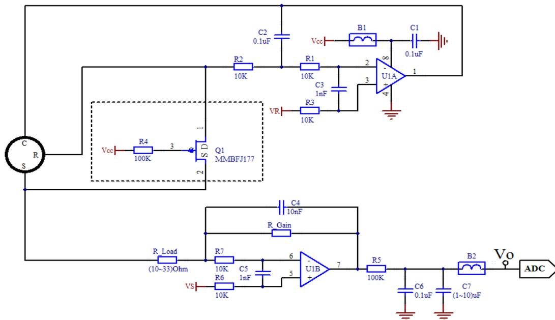
The diagram above is a recommended circuitry for three-electrode EC sensors. It consists of three parts: Potentiostatic Circuit, I/V (current/voltage) Converting Module and Short- Connected Configuration.
